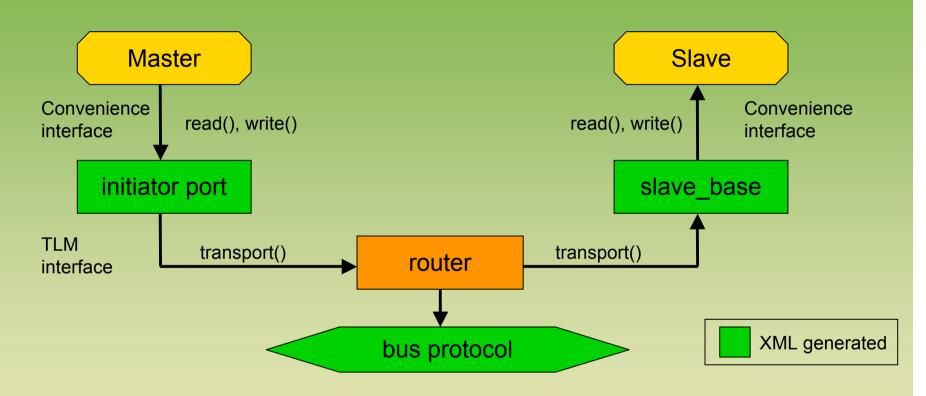
Mixes of abstraction level and protocol are possible, but require wrapper functions which affect simulation performance
